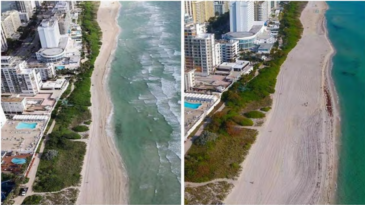
Figure C-2 Beach nourishment before (left) and after (right)
