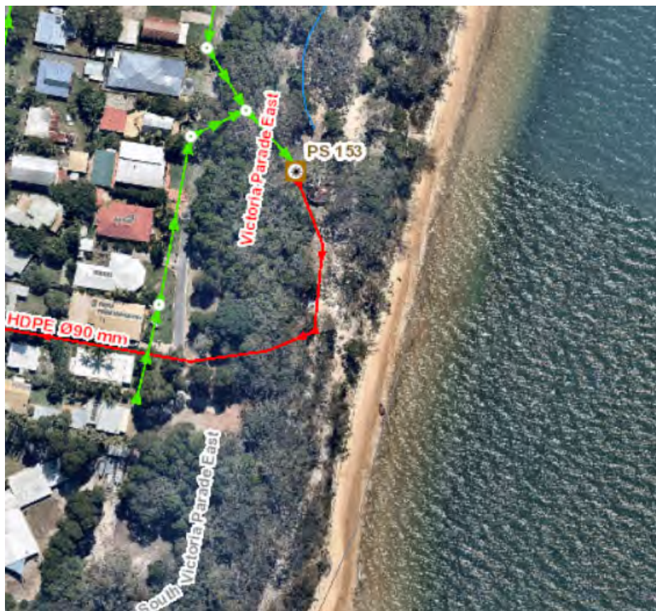
Figure 6-6 Sewer pipe and pump station, Norfolk Beach (Red-e-Map, 2020)
